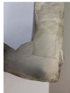
Detail of right side weld – a = 5.5 mm
