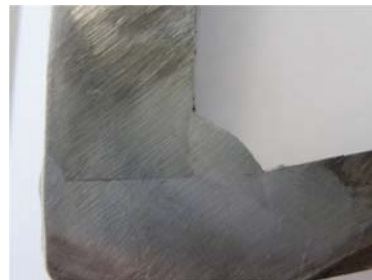
Detail of left side weld – a = 4.7mm
