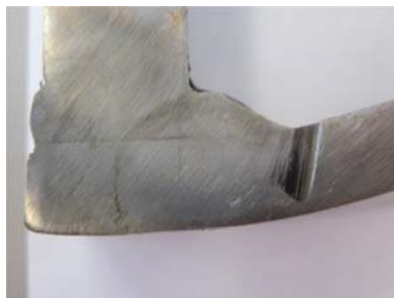
Detail of left side weld – a = 4.3 mm
