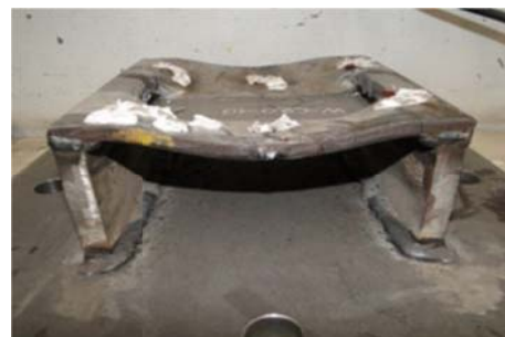
b) test 5 – plate 10mm in compression
