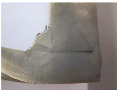
Detail of right side weld – a = 5.5 mm
