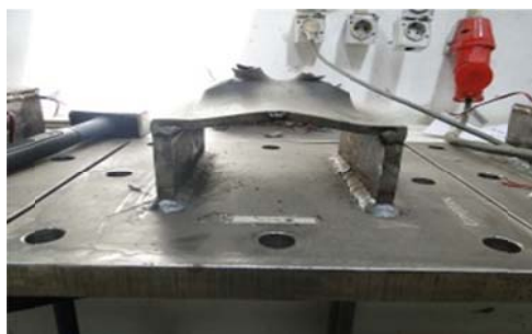
a) test 2 – plate 10mm in tension
