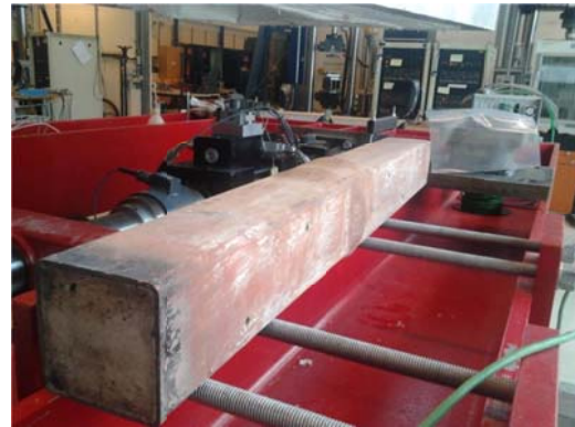
b) Steel-concrete composite SHS column;
